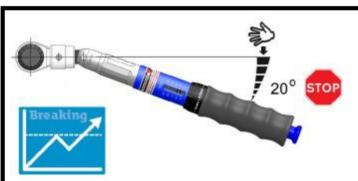
The ATB Wrench is fitted with a reversible square drive ratchet and is designed for use with socket accessories.
